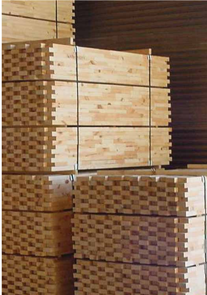
Bundled stacks of finger joint lumber await shipment from the Fort Apache Timber Company's remanufacturing plant at White River, Arizona. Fort Apache Timber Company photo
