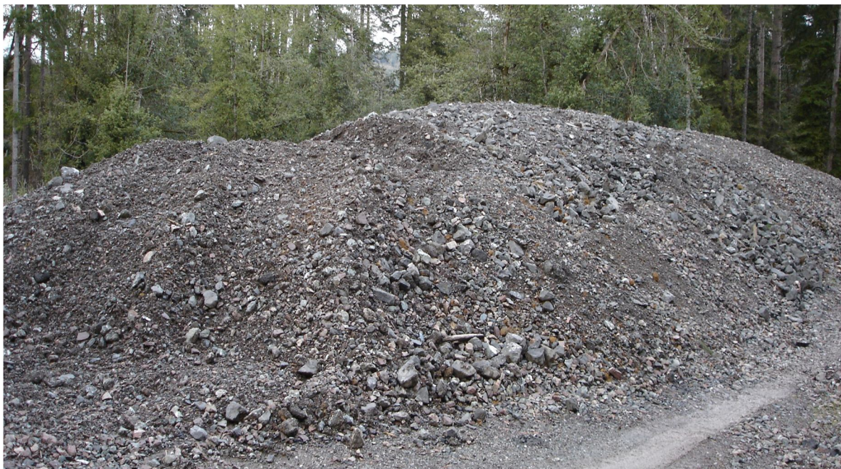
Recycled gravel from road reclamation project – Coquille. Photo by Larry Mason.
