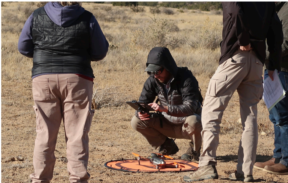
Photo of a trainee conducting a UAS pre-flight checklist, and systems checks per agency standard operating procedure.
